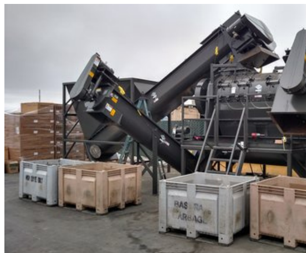
Scott Equipment Turbo Separator machine used in the depackaging process. (Courtesy Innovative Waste Recycling).
